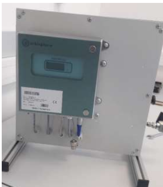
Figure 1 Overview image of the installed hydrogen measurement system
